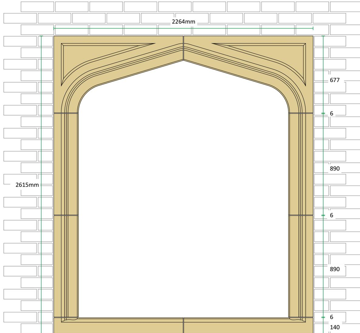
Example Shown to suit 2264mm external width, 1834mm internal width.
